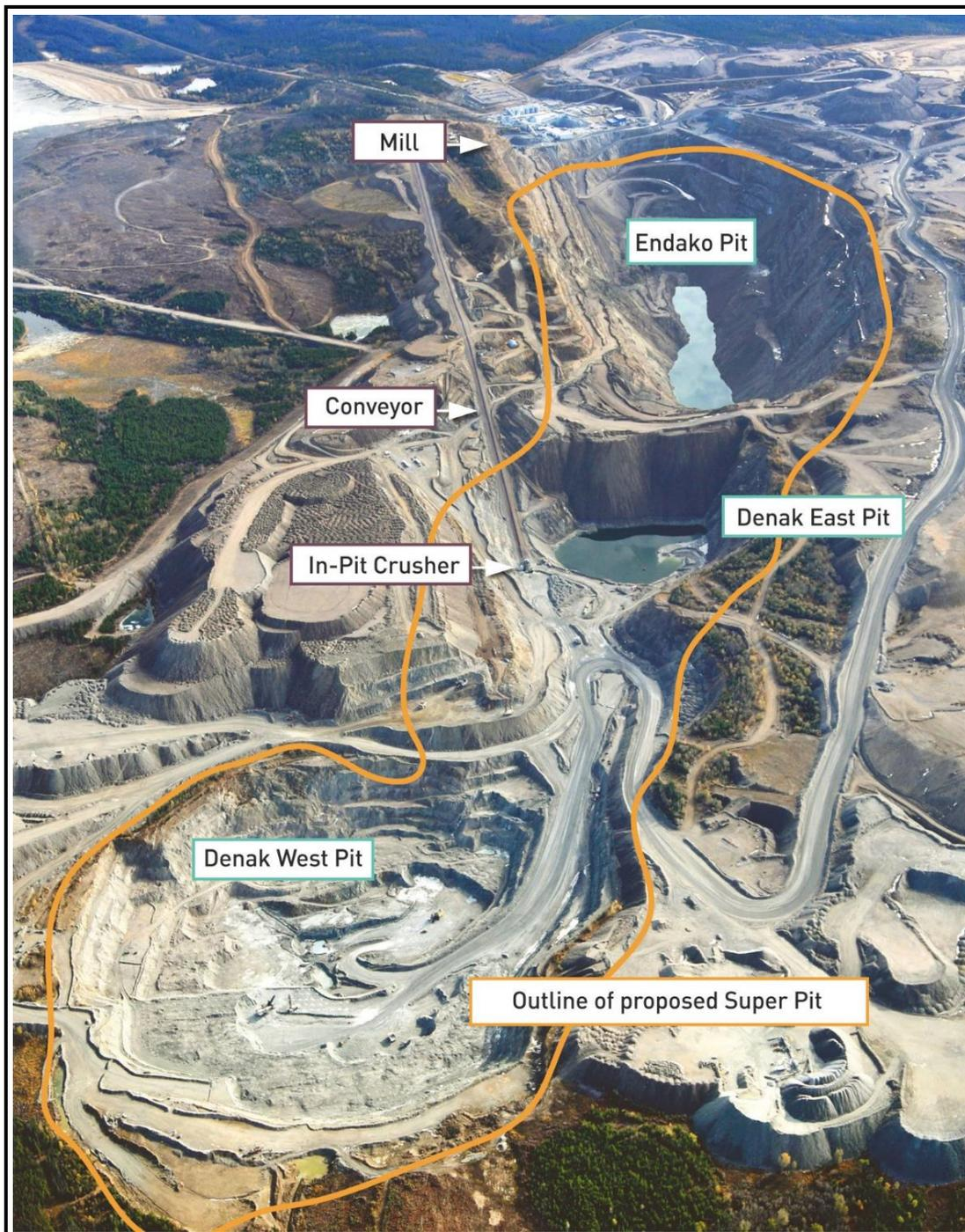
**Figure 2. Aerial view of the Endako porphyry molybdenum mine in central British Columbia, Canada.**
