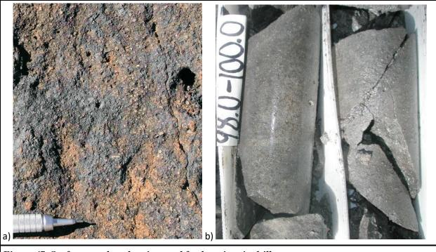
*Figure 47. Surface-weathered greisen and fresh greisen in drill core. Greisen specimens are from the Don Luis tungsten-silver greisen deposit in Sonora, Mexico. a) This weathered surface specimen is dark from a pyrolusite coating because the muscovite is manganese rich. b) Drill core, which is about 6 cm wide, demonstrates that the rock is mainly muscovite with lesser quartz.*
